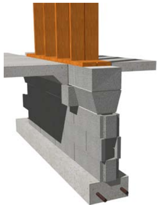
Demising Wall Section with Slab Ledge
